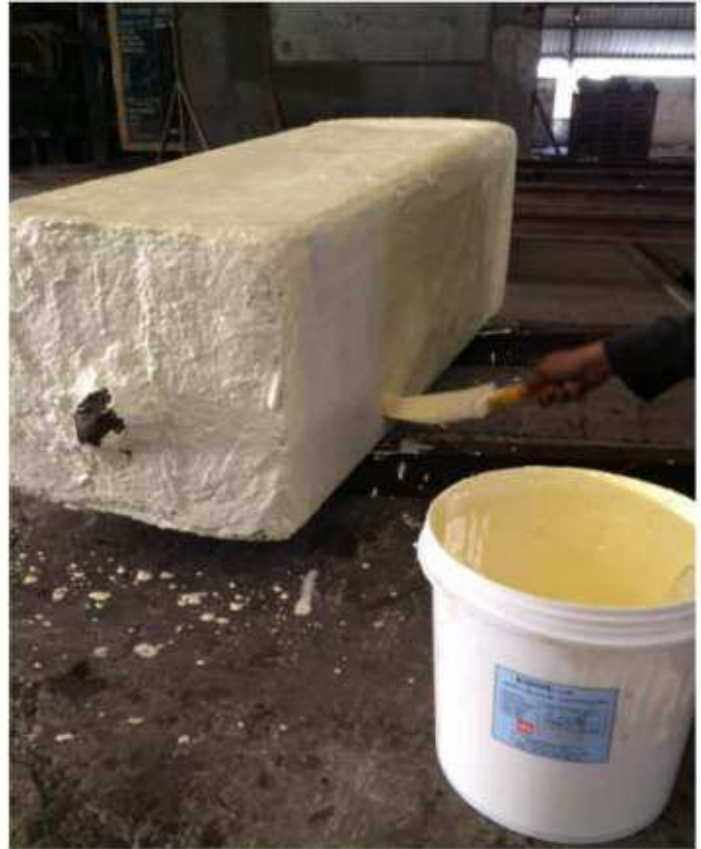
SS-304 ingot coated with ESPON before charging into the furnace.
